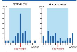
Watanabe Stealth can process with the accurate weight.
