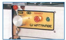
A lever with a safety lock system safely starts the locking system with a equipped emergency stop button.
