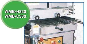
Equipped the crank cover. The crank is covered for preventing meat dusts and the safety. Detatchable, easy to wash, and clean.
